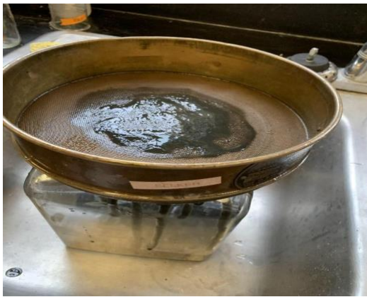
Figure 1. The process of filtering sludge.
